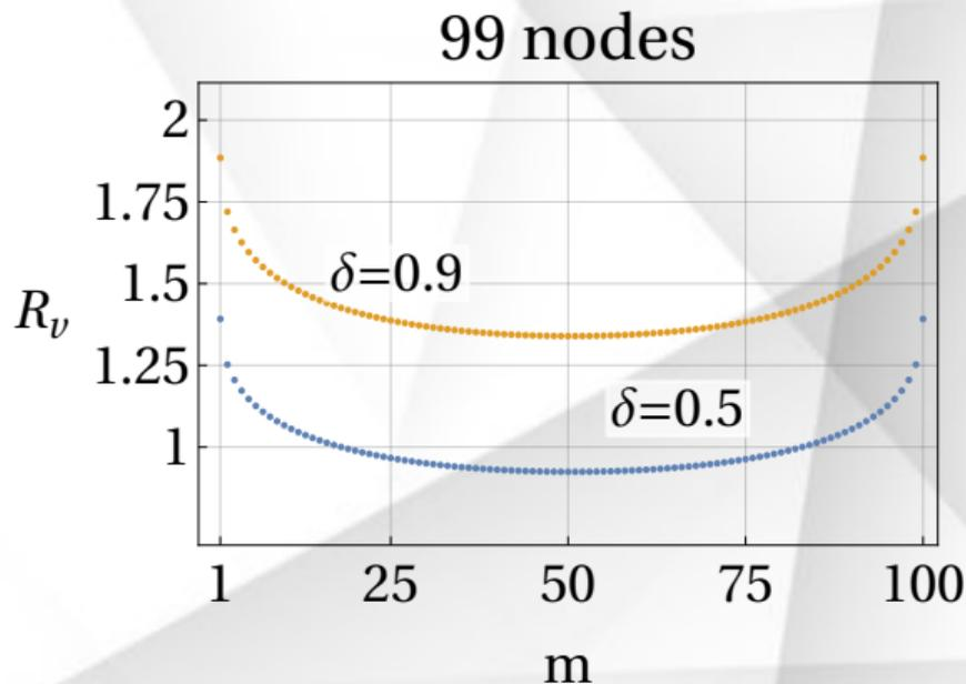
**Figure 2:** Variance in resource consumption with the position of the noisy node  $m$  for the given number of nodes  $n = 99$  and the noise parameter  $p = 0.8$ . This figure is generated for two different values of Schmidt coefficient  $\delta$  of the entangled state in  $\rho(p, \delta)$ . For each case  $\beta = \frac{1}{2}$ .
