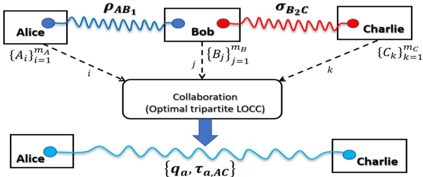
$$F_{AC}^*(\rho_{AB_1}, \sigma_{B_2C}) = \max_{\Lambda \in \text{LOCC}} F(\Lambda(\rho_{AB_1} \otimes \sigma_{B_2C})) > \frac{1}{2}$$
